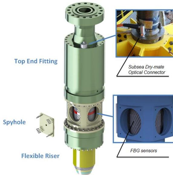
Figure 1 – Spyhole End Fitting with MODA sensors.
