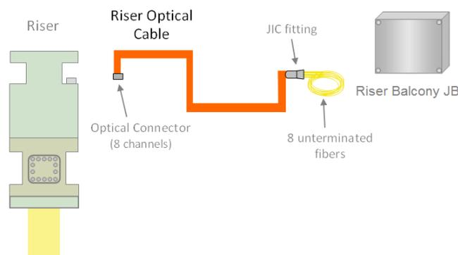
Figure 2 – Riser Optical Cable Schematic.
