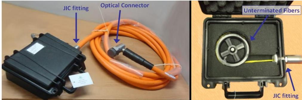
Figure 3 – Riser Optical Cable Picture | Unterminated End Picture.
